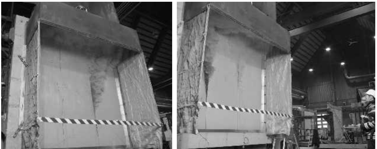
Fig. 7 Panel wall without a free vertical edge: any of the two panel joints (or both) could be seen to release visible smoke; no pattern was observed as to which of the joints will start emitting smoke first
