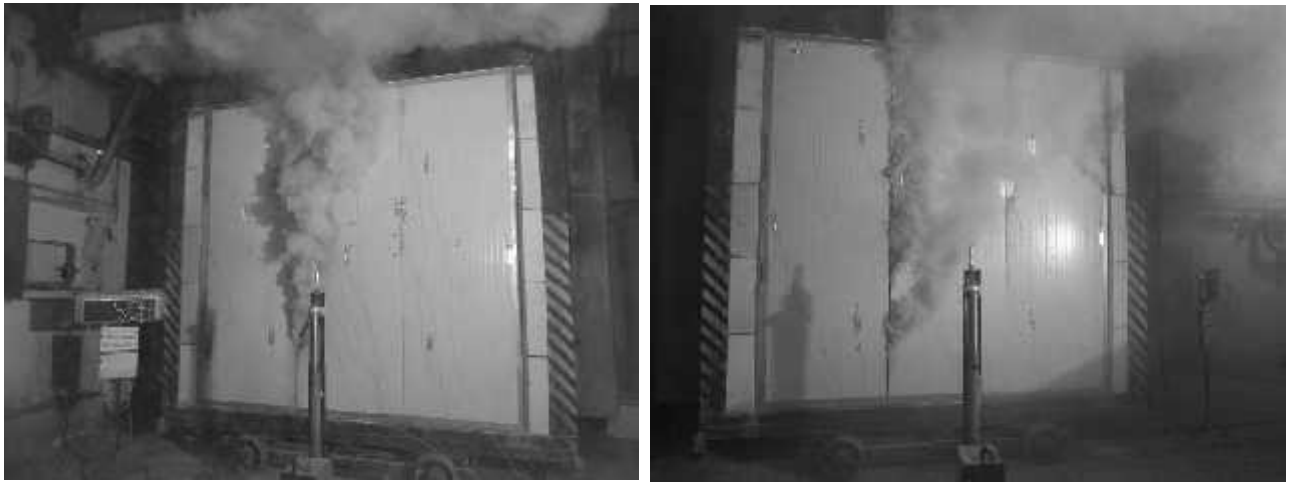
Fig. 6 Panel wall with a free vertical edge: joint placed closer to the free edge was the first to start releasing smoke in all the tests carried out
