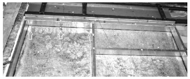
Fig. 6 Additional thermocouples placement in fire resistance test of curtain wall, test 3
