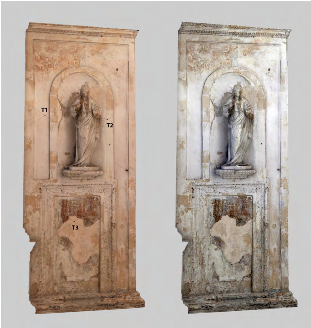
Figure 5: Church of Santo Spirito in Lecce, multiple texture applied on South wall and example of texture replacement using same UVW coordinates with color correct image
