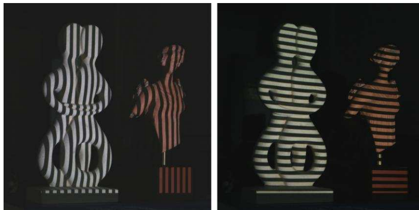
Figure 4: Examples of black and white vertical and horizontal projection patterns.
