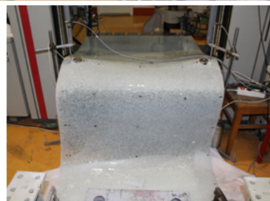
FIGURE 7. Breakdown of the glass railing element.
