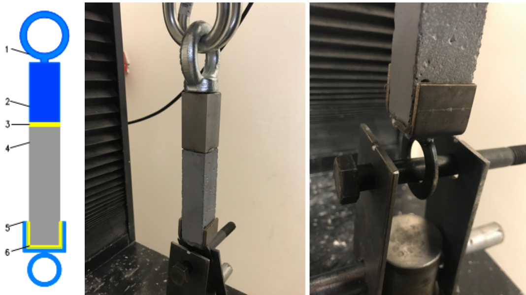
FIGURE 1. Design of tensile test: 1. Steel sleeve, 2. Steel adherent, 3. Selective glue, 4. HPC adherent, 5. Steel sleeve, 6. Construction glue. View on the real specimen in testing machine.
