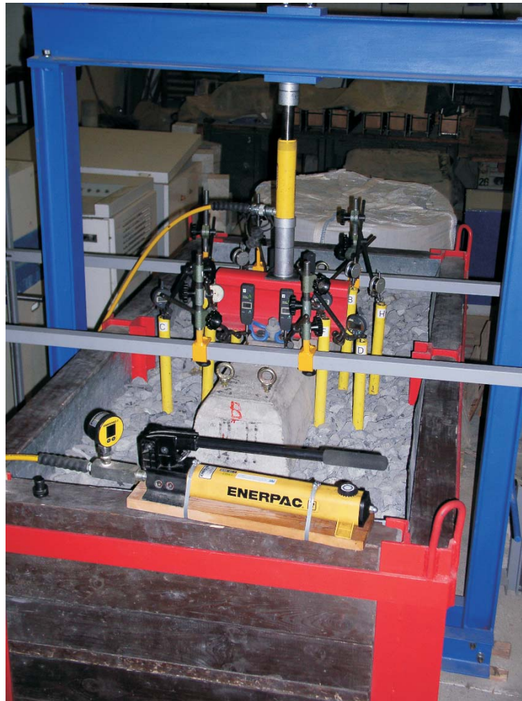
Fig. 6: Deflection measurement due to rail head load
