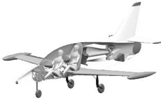
Fig. 2: Accommodation of pilots, engine and fan – 3D CAD model
