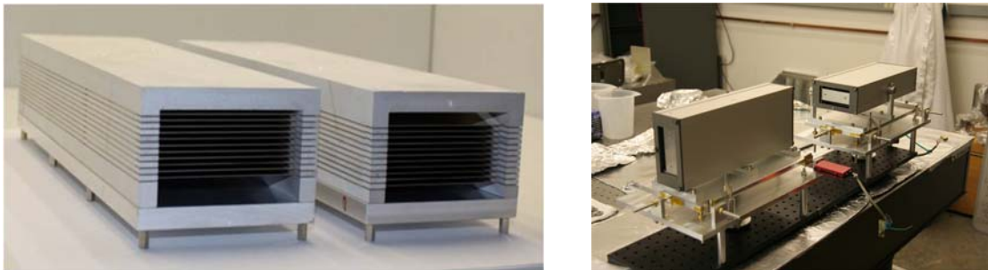
Fig. 6: Left: Test K-B modules assembled in Rigaku RITE in Prague, Right: K-B module during full aperture X-ray tests at Boulder University
