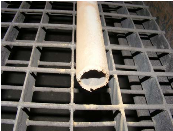
Figure 3: The inlet to the extraction pipe after a one-day test
