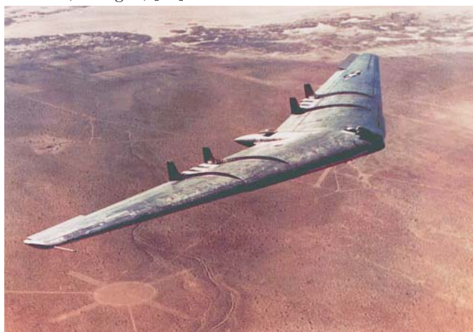
Fig. 7: Northrop YB49 flying wing
