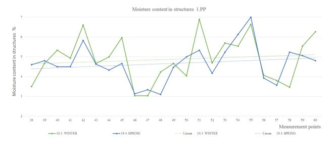
FIGURE 9. Comparison of moisture contents in structures measured in winter and spring – the underground (lower) floor.
