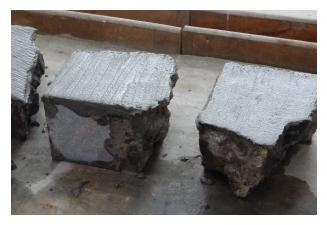
FIGURE 6. Samples with an applied crystallizing coating.
