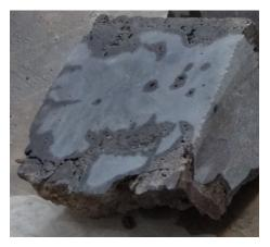
FIGURE 17. Heterogeneous structure on the fracture surface of the sample.
