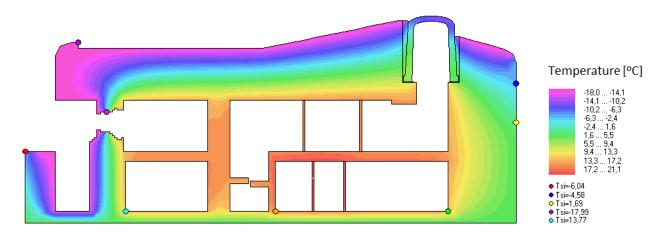
FIGURE 14. 2D thermal performance model of the cross-section (Area 2017).
