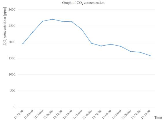
FIGURE 15. Measured values of carbon dioxide concentrations in the dormitory room.
