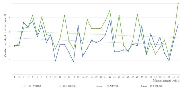
FIGURE 8. Comparison of moisture contents in structures measured in winter and spring – the first (upper) floor.
