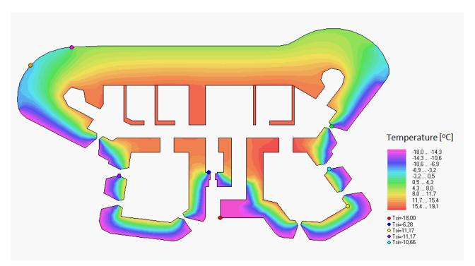
FIGURE 12. 2D thermal performance model of the first floor (Area 2017).
