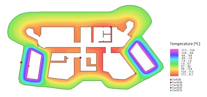
FIGURE 13. 2D thermal performance model of the underground floor (Area 2017).
