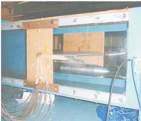
Fig. 5: Model installation inside the wind tunnel
