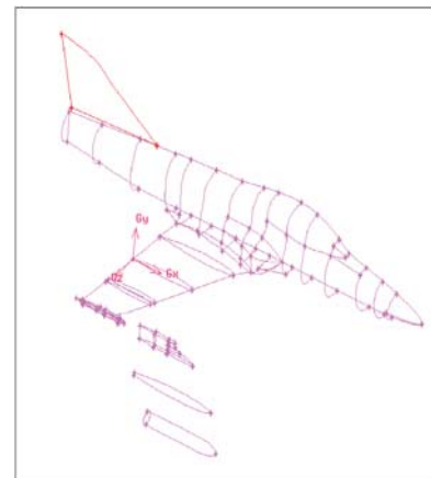
Fig. 3: Digitized wing geometry smoothed with the use of CAD
