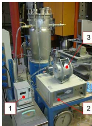
B – part of the biogas yield investigation 1 – cooling, 2 – gas analyser, 3 – flow meter
