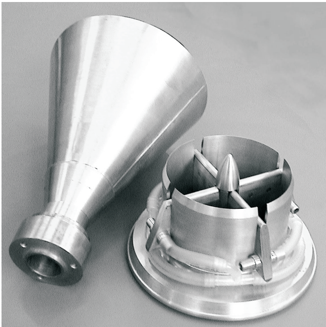
Fig. 8: Actual nozzle (left) and swirl generator (right) used in the experimental investigations
