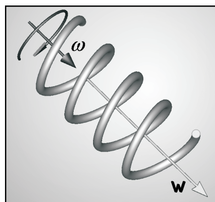
Fig. 1: Helical deformation of a fluid volume in turbulent flows. This idealised shape would arise in the exceptional case of strong rotation with mutually collinear vorticity and velocity vectors.
