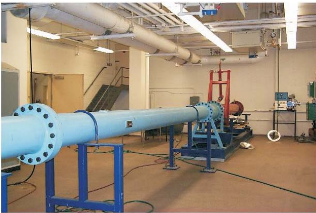
Fig. 1: Shock tube facility at CCNY, Driver section
