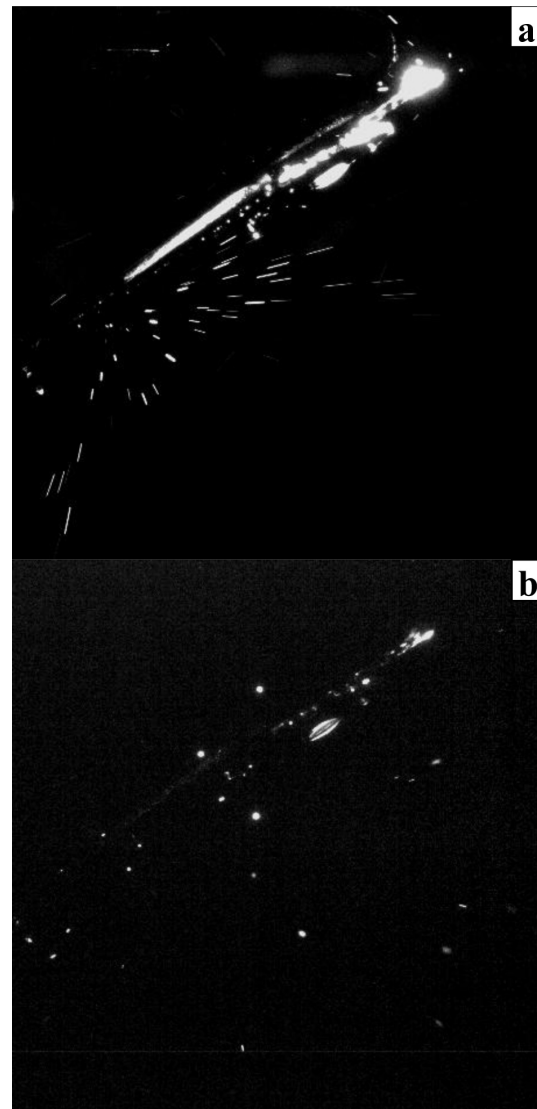
FIGURE 2. High speed images of plasma interaction with inclined ( 35^\circ to plasma jet) tungsten target, a) t = 1.16 ms and b) t = 9.06 ms after the start of plasma-surface interaction, Q_{\text{surf}} = 0.75 \text{ MJ m}^{-2} , t_{\text{exp}} = 0.25 ms.
