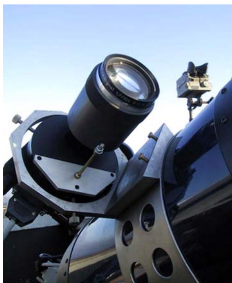
Fig. 1: OMC Test Device (providing real test images) operated at AI Ondrejov prior to the launch of INTEGRAL. BART Wide Field CCD camera, FOV 6 \times 7 degrees, lim mag 15.5, identical with INTEGRAL OMC Test Device (18 arcsec/pixel)
