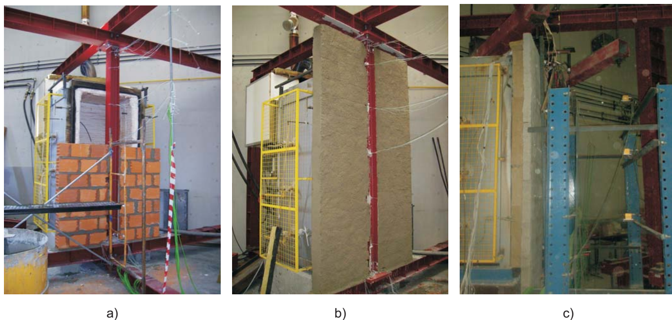
Fig. 2: a) Construction of the test model, b) Column embedded in the wall, c) Lateral view of the experimental system
