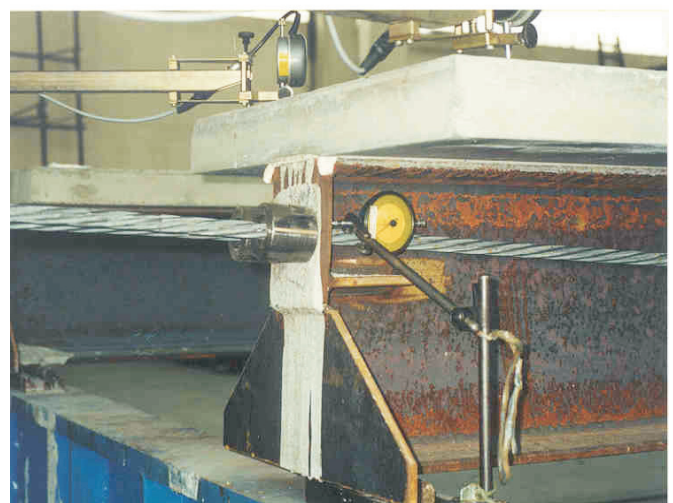
Fig. 4: Structural detail at the end support section showing the head of the anchorage device acting against a rigid steel plate
