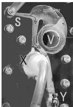
Fig. 7: Visualised flow in the model valve in its OPEN state. Clearly recognisable due to the condensation is the spill-over flow into vent V. Its magnitude can be estimated.
