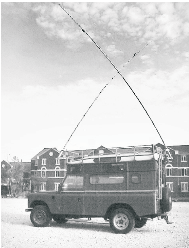
Fig. 12: Vehicular mounted shortened DM aerial, inductively loaded, has narrow SWR bandwidth but can be tuned readily with an ATU. Its potential for NVIS in fieldwork is being currently investigated
