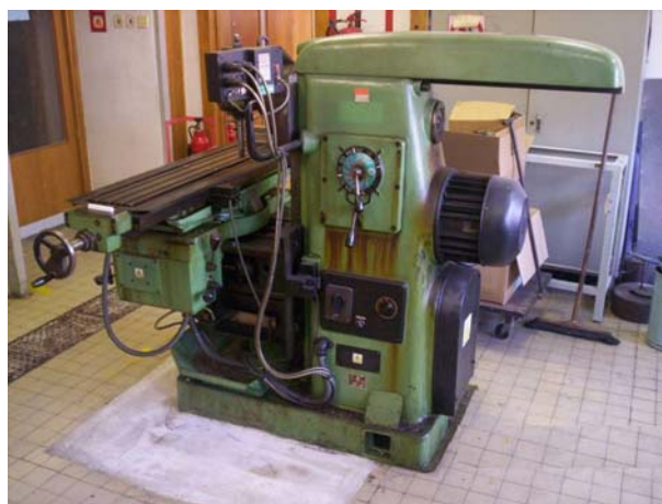
Figure 1: Tested milling machine with a vertical spindle — side view [3]
