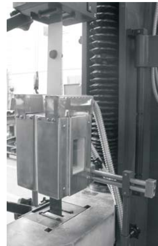
Fig. 2: Electric furnace for the tests in 2007
