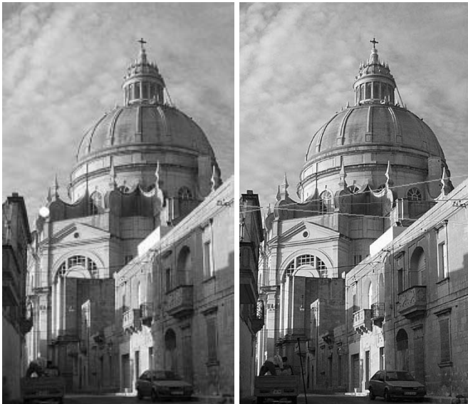
Fig. 1: Envelope of epipolar lines: We computed the epipolar line (dark) and the epipolar band (light) in the second image. The point in the first image that we used for the computation is marked by a white point. The epipolar band shown here represents the envelope of epipolar lines with equal k^2 = 5.99915 . The according probability that the true epipolar line lies within this band is \alpha = 0.95 . We see that for this value the conic is a hyperbola with two branches.
