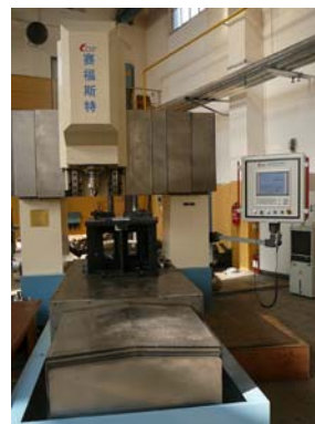
Figure 2: FSW – LM-060 welding equipment
