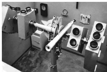
Fig. 1: (Left) The cluster of sky patrol photographic cameras operated in the Boyden Observatory, South Africa, by the Bamberg Observatory. (Right) The Bamberg Zeiss blinkmicroscope and the Southern Sky Patrol Plates
