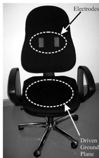
Fig. 1: The “Aachen SmartChair”: A single lead cECG system in an office chair [10]
