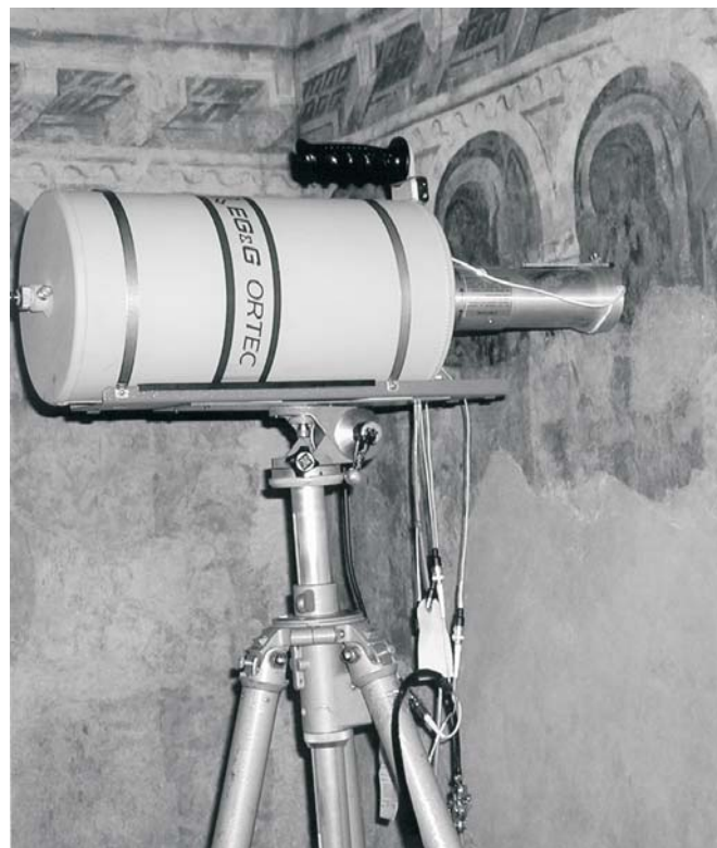
Fig. 1: Si(Li) detection equipment during the measurement of a fresco
