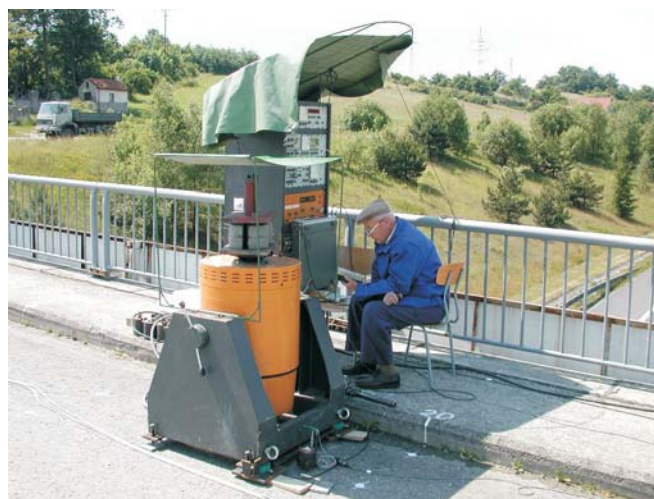
Fig. 7: The TIRAVIB 5140 electrodynamic exciter and its placement on the bridge
