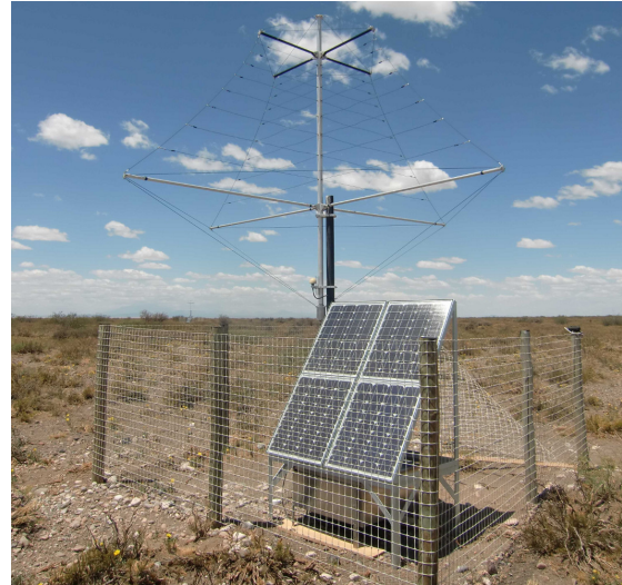
FIGURE 2. Photograph of an AERA radio-detector station.
