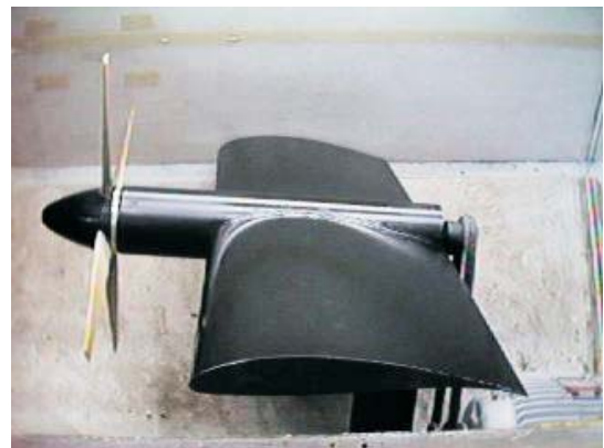
Fig. 4: Tractor propeller model
