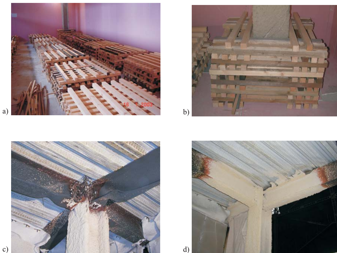
Fig. 1: a) Fire load in compartment; b) fire load around column D2; c) protection of internal column D2 (after test), d) protection of external column (after test)
