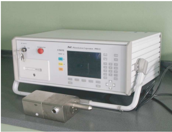
Figure 1. The PRS400 Photon Radiosurgery System consists of the X-Ray source and the control console
