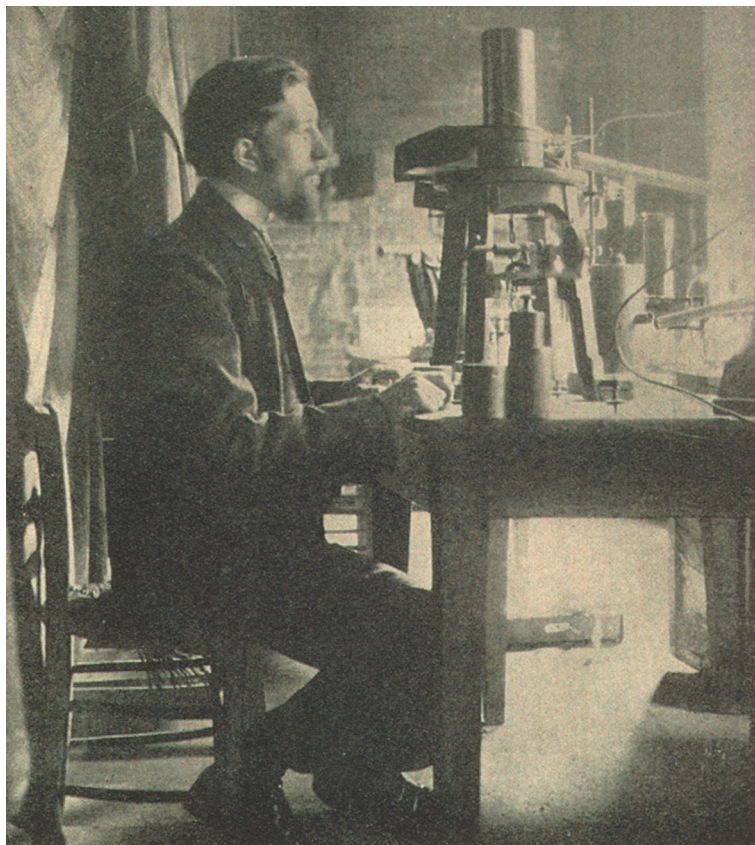
Figure 10. Pierre Curie using a quartz piezoelectrometer. This photograph is one of the few published in the biography of Pierre by Marie Curie. It is probably the only now existing side-view image of Pierre using this device [1]. All others, such as Figure 11, are frontal views
