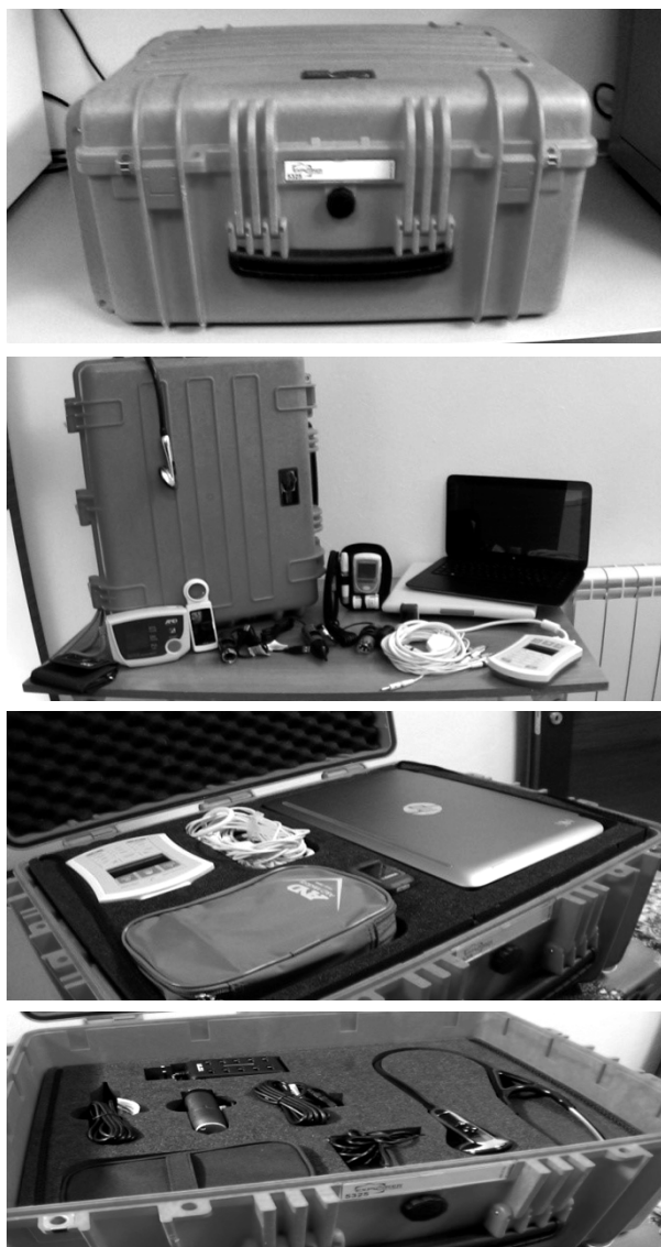
Figure 11. Telemedicine case already installed or being installed in 2015 on board of 50 ships belonging to the French company CMA Ships in Marseille. The case contains an artificial intelligence system for helping to prepare a more precise request for medical advice [24] and the telemedical devices listed below: infrared thermometer, high quality photocamera, electronic phonendoscope, blood pressure monitor, 12 derivations electrocardiogram, spirometer and SPO2, glucometer
