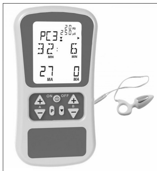
Figure 4. Electrostimulator with a rectal electrode used in biofeedback therapy for faecal incontinence
