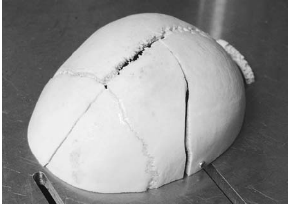
Figure 3. Example of fractures created following compression forces applied to the vertex of the isolated calvaria. The first fracture was the parietal bone fracture. Diastases of the sagittal and lambdoid sutures occurred next, followed by fracture of the frontal bone.
