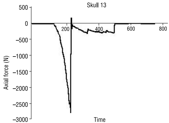
Figure 7. Graphical examples of an isolated calvaria (specimen 13, Fig. 4) following the application of compressive forces to the vertex. The initial fracture occurred at 2700 N.
