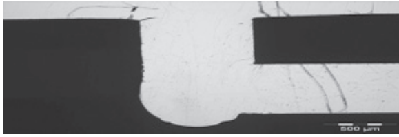
Figure 3. Form drill (Camlog®, diameter 4.3 mm, length 11 mm, internally cooled). Thin-section 2.5 \times showing the cooling channel port.
