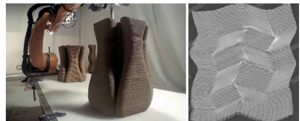
Figure 5. A robotic 3D print fabrication at IAAC (IAAC, n.d.) and a material study at Bauhaus (Albers, 2014).
