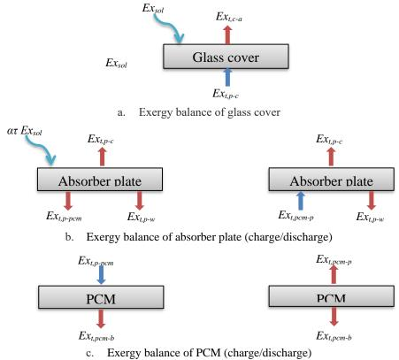
Figure 2. Exergy balance of the solar collector components.
