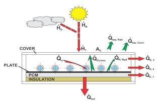
Figure 1. Heat transfer terms involved in solar collector.
