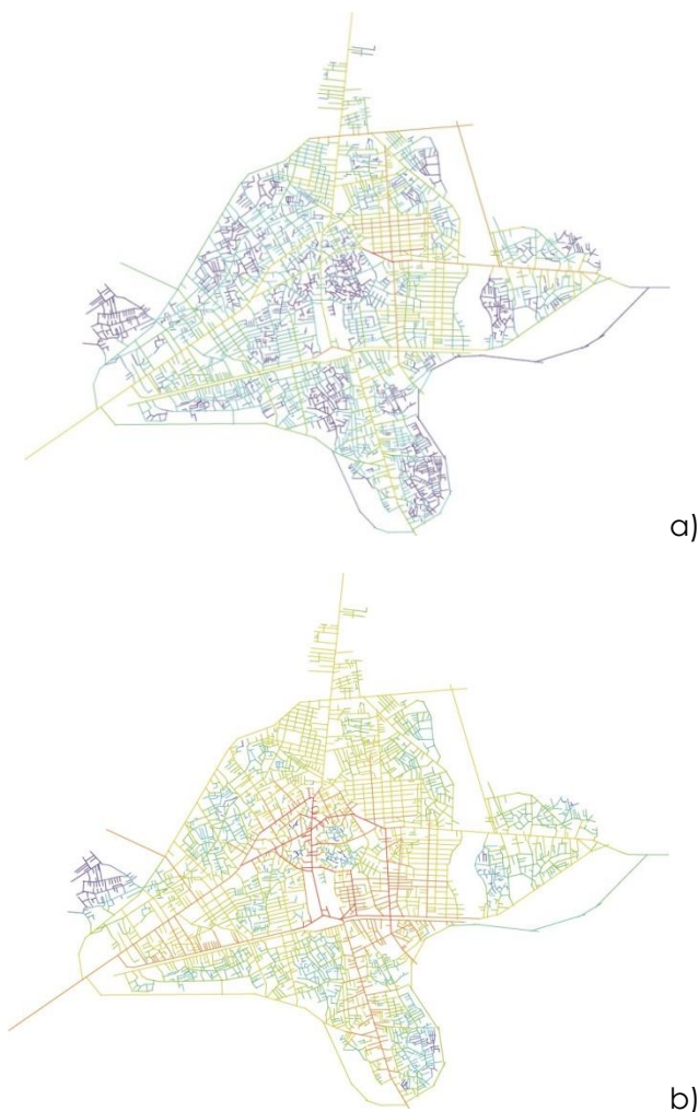
Figure 4. Urban road total depth of future plan in scale R5 (a) and R10 (b)
