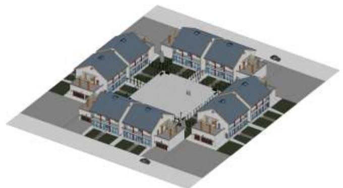
Figure 26. Beijing new courtyard garden house compound based on a system of 78 m × 78 m standard block size, the
