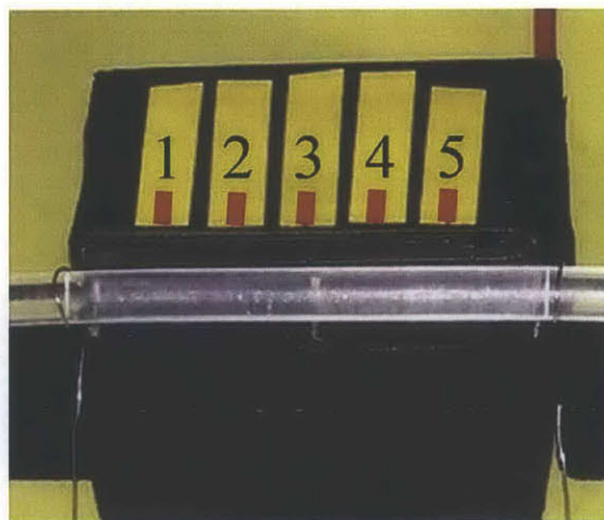
Figure 5.9. A pixelated H8500 PMT was used to measure the distribution of light escaping the side of a FEP tube. The top row of a H8500 PMT consists of eight pixels. ^{90}\text{Sr} pulse height spectra are collected from each pixel for the source placed at the five location identified.
