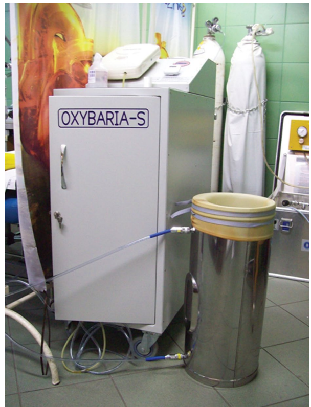
Figure 4. The apparatus OXYBARIA-S for local hyperbaric oxygen therapy interventions (manufactured by FASER S.A., Poland)
