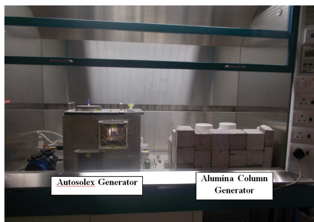
Figure 8. Autosolex Generator occupying 0.88 sq. m area inside fume hood
