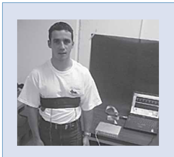
Figure 1. Recording of electrocardiogram signals from capacitively-coupled, non-contact sensor (CCNS) through a cotton T-shirt.
