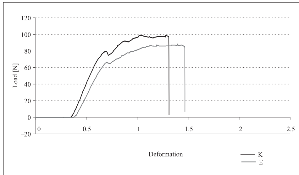
Figure 1. Typical load-deformation in the femur shaft bending three point test in the groups of animals; K — control group; E — pregnant females with caffeine applied
