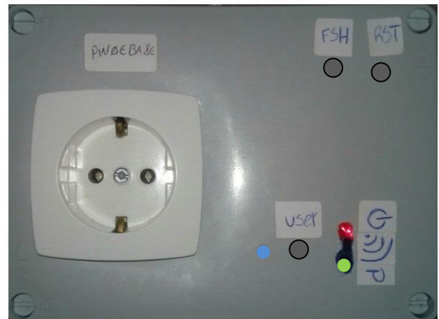
Figure 4 - Frontal panel and user interface of the EG-Plug
