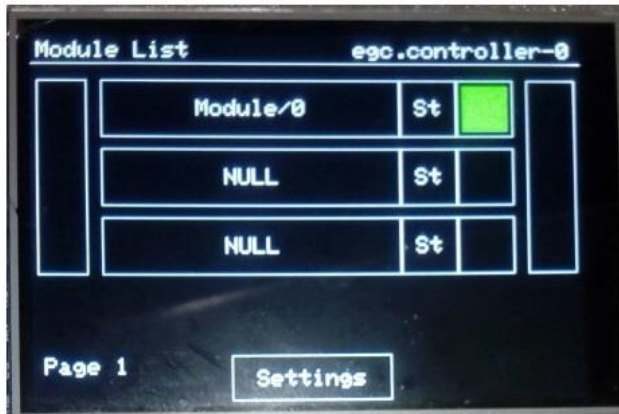
Figure 8 - Controller's Module (EG-Plug) list
