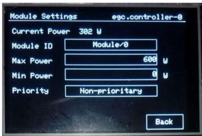
Figure 9 - Controller's Configuration menu for a specific EG-Plug
