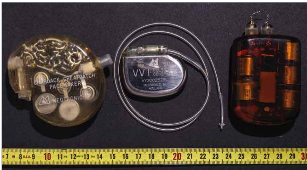
FIGURE 3: An early Chardack Greatbatch pacemaker from the 1960s contrasted with a modern single chamber unit with bipolar tined transvenous electrode.
